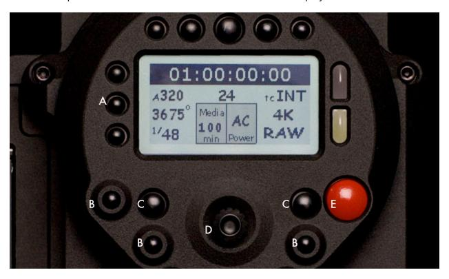
A - Quick Access Access to Exposure, White Balance and Shutter Speed
