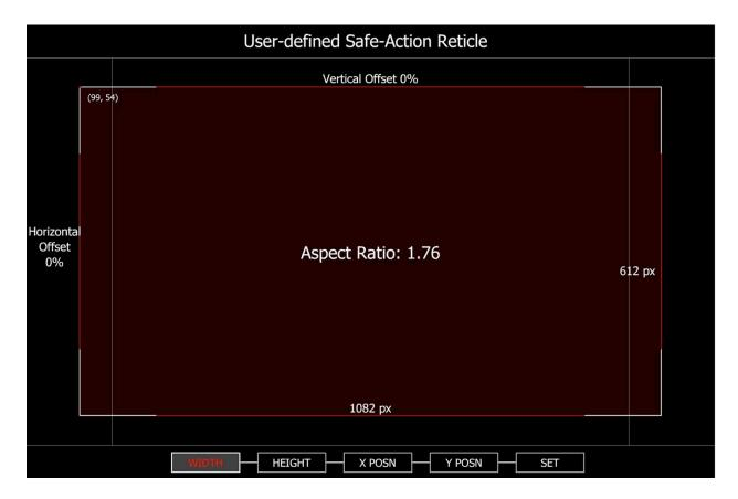
**X POSN:** Adjusts the horizontal center position of the guide.
