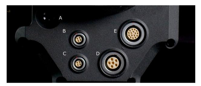
A Power On/Off switch B Aux Power / GPIO A
