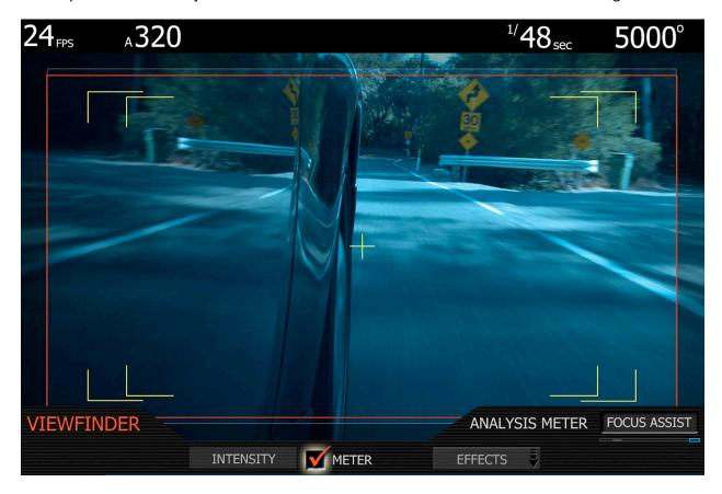
System information including instantaneous frame rate, sensitivity, shutter speed, color temperature, recording format, clip name, timecode, battery and media remaining is provided in the RED-LCD or RED-EVF monitor outputs, and the rear status display on the camera back.
