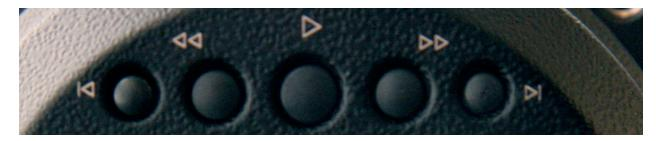
The I> key is used to enter PLAYBACK mode, and to initiate playback of the last recorded Clip. Press it once to enter Playback mode, and a second time to start playback. Once in clip playback, this key acts as a Play/Pause toggle.
