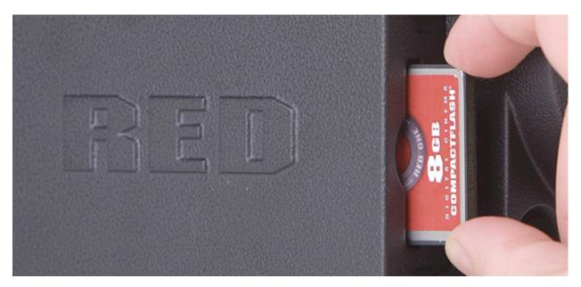
Inserting a Compact Flash card
